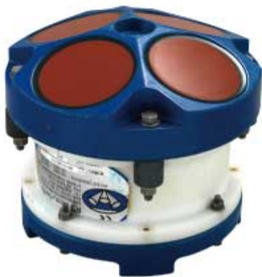
① 음향도플러유속계 ADCP(Acoustic Doppler Current Profiler)
